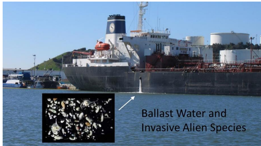
Figure 5-2: Ballast Water Release
